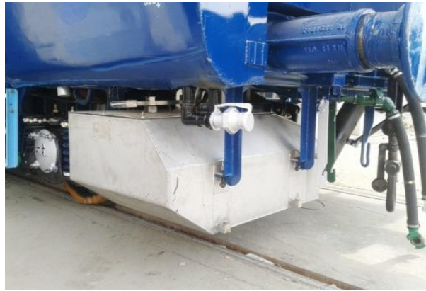
Img: Bio toilet str Fixed in ICF Coach
